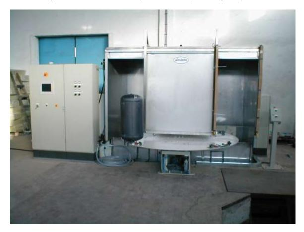
The system, which has two application stations and may be operated by one person, has a typical production of 30 to 40 boilers of 80 liters per hour, depending upon the product complexity & application requirements.
